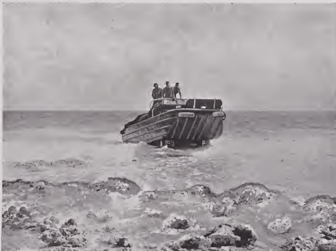
FIGURE 107. Using 30-pound tire pressure, DUKW negotiates coral reef in tests at Funafuti.
